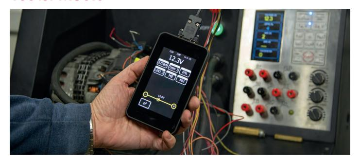
**Tester MS016** is a compact multifunctional device for express diagnostics of the following automotive units without removing them from vehicles: 12/24V alternators, 12V alternators for Stop-Start systems, and starters. The tester deterimines the performance of voltage regulators - separately from alternators, and it also reads and saves data transmitted via a vehicle LIN bus.
