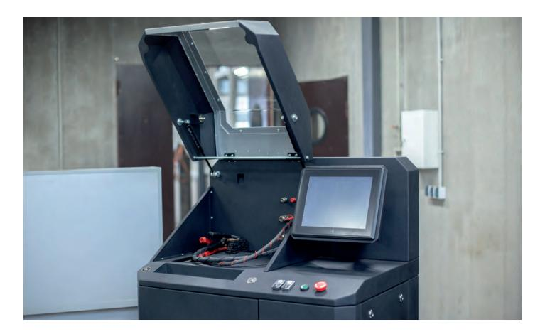
**MS005** – multifunctional test bench designed for the quick and the accurate diagnostics of the automotive alternators and starters of the passenger cars and the trucks. The test bench software is regularly updated for the expanding of the range of diagnosed units.
