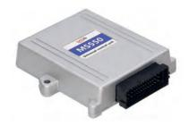
Adapter MS550 is designed for a joint usage with tester MS561 to test electric power steering racks without control units (mainly in Japanese vehicles). The adapter is an accessory tool for diagnostics of both electric (electric motor, electric motor position sensor, torque sensor) and mechanical parts of a steering rack with tester MS56. It can be also used for a torque sensor calibration.
