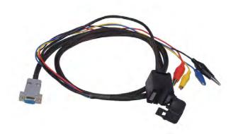
**Tester MS016 and cable MS-33503**, we can register both: a voltage across starter terminals 31, 30, 50, 45 and a current across terminal 30 during the engine start. The measured parameters are displayed on the tester screen as diagrams. In addition, the maximum and minimum values are displayed numerically. This information helps recognize problems with the starter, battery, or wiring.
