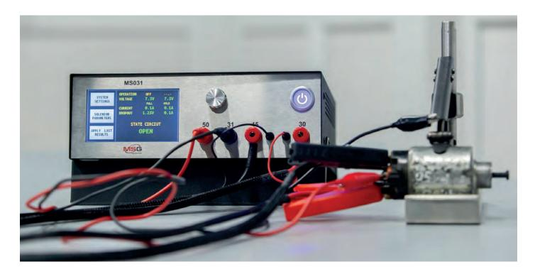
**Tester MS031** is designed for checking of the technical condition of starter solenoids and detection of open-circuit and short-circuit faults in solenoid coil.
