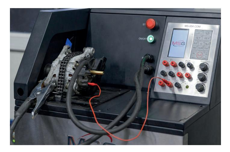
**Test bench MS004 COM** is used to determine the technical condition of the following automotive units: alternators under different loads (100A for 12V, 50A for 24V), 12/24V starters with the power of up to 4kW, and voltage regulators of the latest models. Technical parameters of the test bench allow the detection of 99% of potential alternator problems. The test bench allows to also make a proof test of an electrical unit after its repair.
