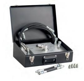
Tester MS611 is designed for a checking of hydraulic power system elements - steering racks and pumps without their dismantling from a vehicle. The tester determines the technical condition of the units and the necessity of their dismantling from the vehicle for the further repair.
