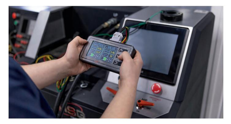
**Tester MS121** is a compact device that combines two functions: testing of electromagnetic clutches and control valves of automotive climate system compressors.
