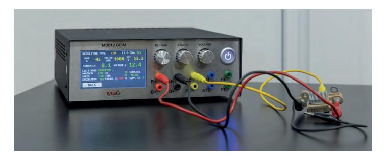
**Tester MS012 COM** simulates the connection of a voltage regulator to a properly operating alternator to determine its performance and to select the regulator analogue for a specific alternator.
