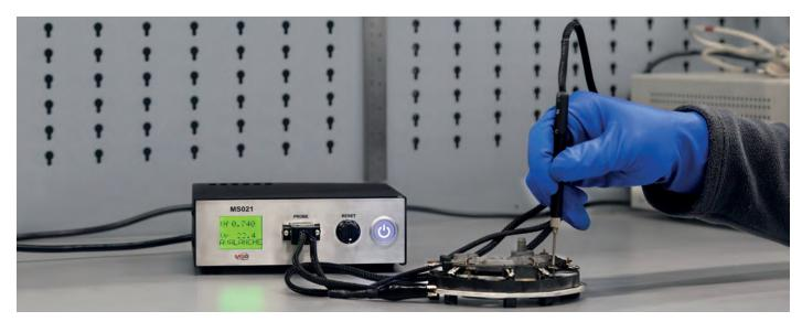
**Tester MS021** ensures accurate testing of the technical condition of alternator diode bridge and a single diode. The tester identifies the type and performance characteristics of a tested diode, reports on the defect type and identify the diode degradation.
