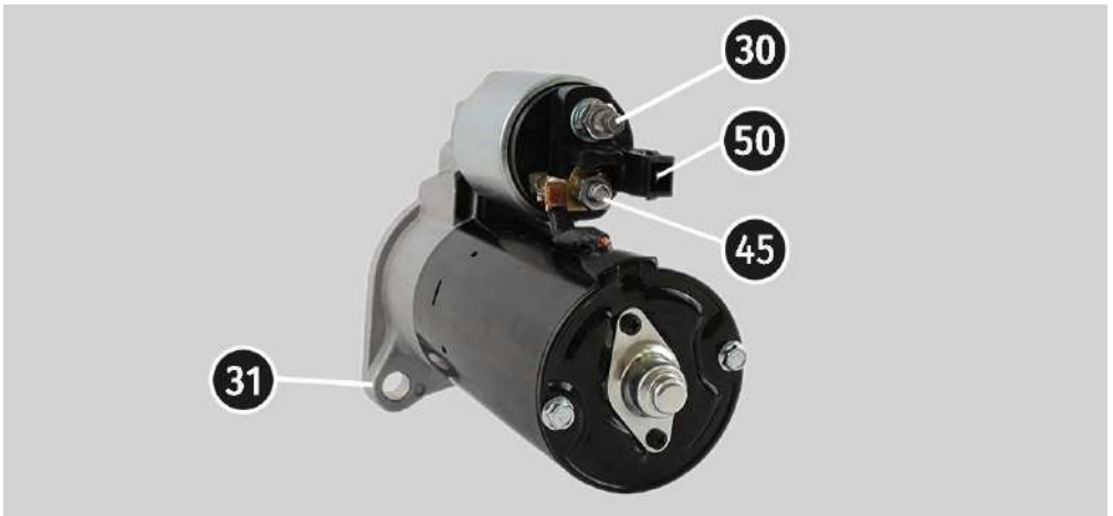
Figure 20. Position of terminals on the starter.
