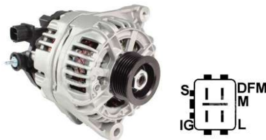
Figure 13. Toyota 2706020230 alternator and connector terminal references.
