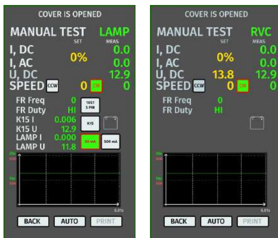
Figure 7. Test menu for alternators LAMP and RVC type
