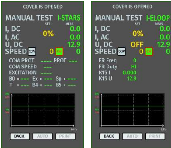
Figure 11. Test menu for alternators I-STARS and I-ELOOP type
