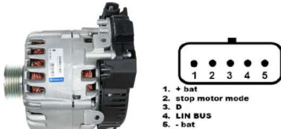
Figure 25. Alternator Valeo IST60C017 and connector terminal references
