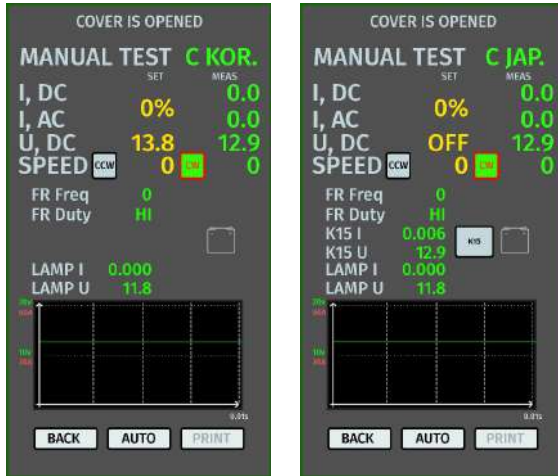
Figure 8. Test menu for alternators C KOR and C JAP type
