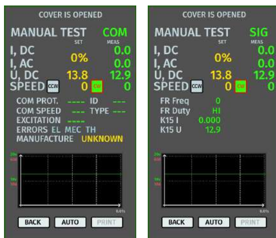
Figure 10. Test menu for alternators COM and SIG type
