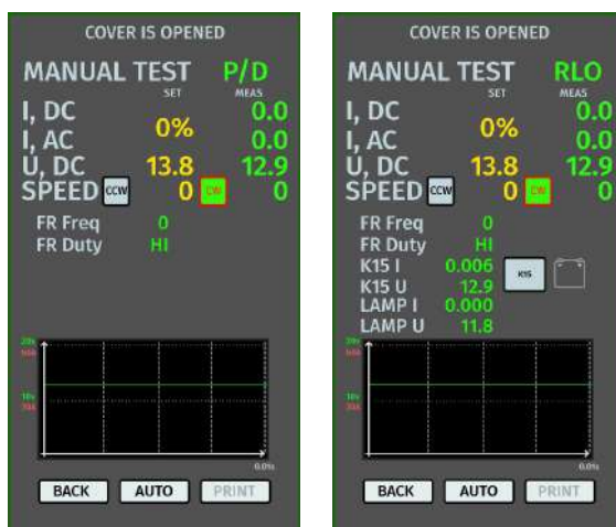
Figure 9. Test menu for alternators P/D and RLO type
