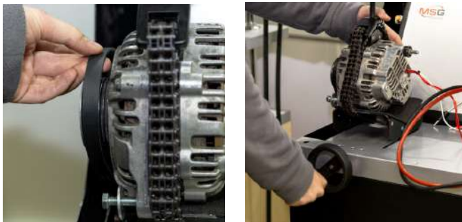
Figure 16. Installation of the belt to the alternator pulley
