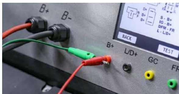
Figure 24. Connection of two wires to the test bench output
