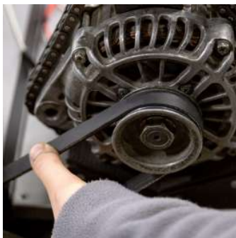
Figure 17. Belt tightness check
