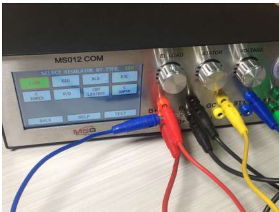
Figure 19 – Connection of additional cable B+
