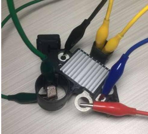
Figure 16 – Voltage regulator ARE1054 connected to the tester output terminals
