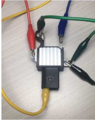
Figure 21. Voltage regulator ARE6149P connected to the tester terminals
