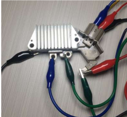
Figure 18 – Diagram of voltage regulator ARE6076 connection to the tester
