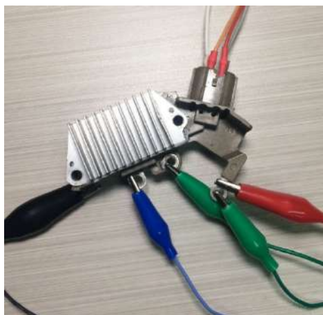
Figure 14. Voltage regulator ARE6076 connected to the tester terminals
