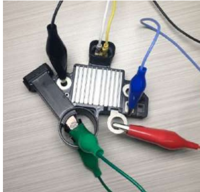
Figure 12. Voltage regulator ARE1054 connected to the tester terminals
